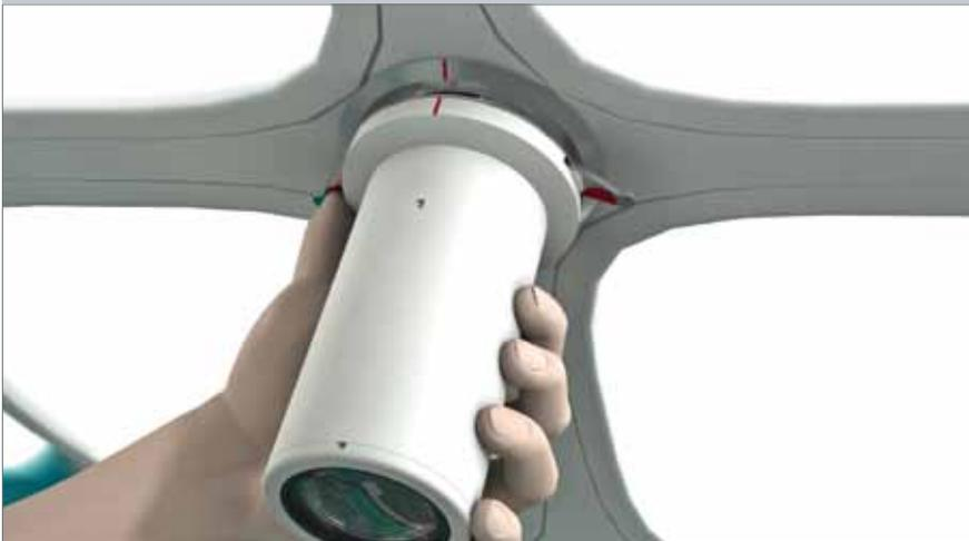
Simply insert the Vidi OP camera in the Vidi OP socket, and the contact for signal transmission has been made. Fasten the safety levers, and the job is done.
