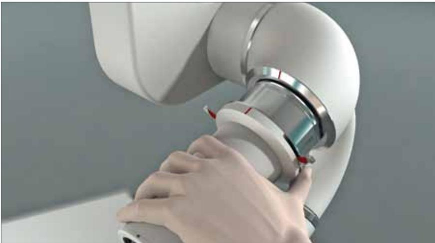
Unfasten the safety levers and the Vidi OP camera is ready for a fast move.
